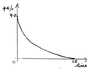
(11) This increases the time to charge. The larger resistance reduces the changing current, hence the time taken for a fixed amount of Charge to build up on the plates is increased 9 = It
