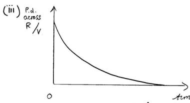
(b) The discharge time is less than the charging time. Since the capacitance is the same the discharge Moistance must be smaller than the charging Moistance.
