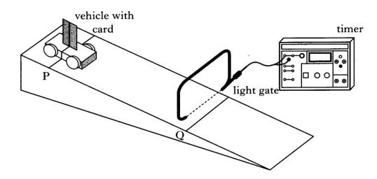
The line on the trolley is aligned with line P on the track.
