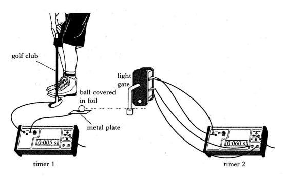
The club hits the stationary ball. Timer 1 records the time of contact between the club and the ball. Timer 2 records the time taken for the ball to pass through the light gate beam.
