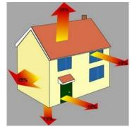
In our homes we lose heat energy through the walls, through the roof, through the floor and through windows and doors.
