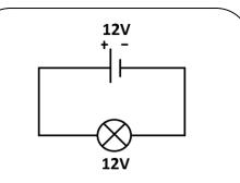
In this case the electron passes through the battery picking up 12 bits of energy. It then goes through one light bulb, giving all of its energy away. The bulb is 3x brighter in this circuit as it gets 3x more energy per electron passing through.
