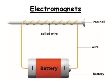
An electromagnet is a type of magnet which only becomes magnetic when an electrical current flows through its coils.
