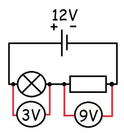
In this circuit the battery gives out 12 bits of energy to every electron (12V). When an electron moves round the circuit and passes through the resistor it loses 9 bits of energy. It then passes through the bulb and loses its last 3 bits of energy. As it has no energy left it needs to go back to the battery to get more energy and the cycle repeats.
