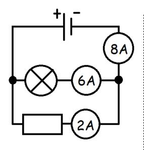
The ammeter closest to the battery is 8A, meaning 8 electrons are whizzing through it every second.
