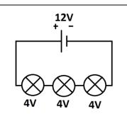
In this case the electron passes through the battery picking up 12 bits of electrical energy. It then goes through three light bulbs. At each one it gives away 4 bits of energy. By the time it passes through the bulbs it has no energy left, so it goes back up to the battery to get more energy. Then the whole process happens again.
