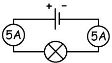
In this circuit the current is 5A at all points. This means 5 electrons whizz passed every second. So when 5 electrons pass through the battery in one second then another 5 electrons are passing through the light bulb in the same second. No matter where you look in the circuit you would see 5 electrons going passed every second.
