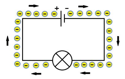
To do this we use a very special device to count how many \_\_\_\_\_\_ are going passed every \_\_\_\_\_. The device is call an ammeter. The units we use to measure current are called amperes, but usually we call it amps or A for short.
