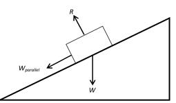
W is the weight of the object and R is the reaction force acting perpendicular to the slope. If we draw these two forces tip to tail as described in section 1.1 we get the resultant force  $W_{parallel}$  shown in the diagram below.
