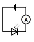
In **photoconductive** mode the photodiode is connected in reverse bias with a cell. No current will flow in this mode but when light is shone on the photodiode electron hole pairs are created which causes a current to flow. Current and irradiance are proportional.
