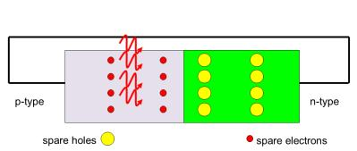
In a photodiode photons incident on the junction region cause electron-hole pairs to be created and a current to flow.
