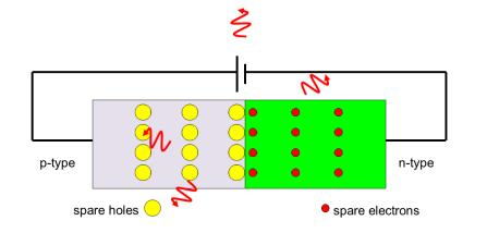
In an LED the applied Voltage lifts electrons into the conduction band from the valence band. The electrons then fall from the conduction band and combine with holes in the valence band and to conserve energy a photon is emitted from the junction region.
